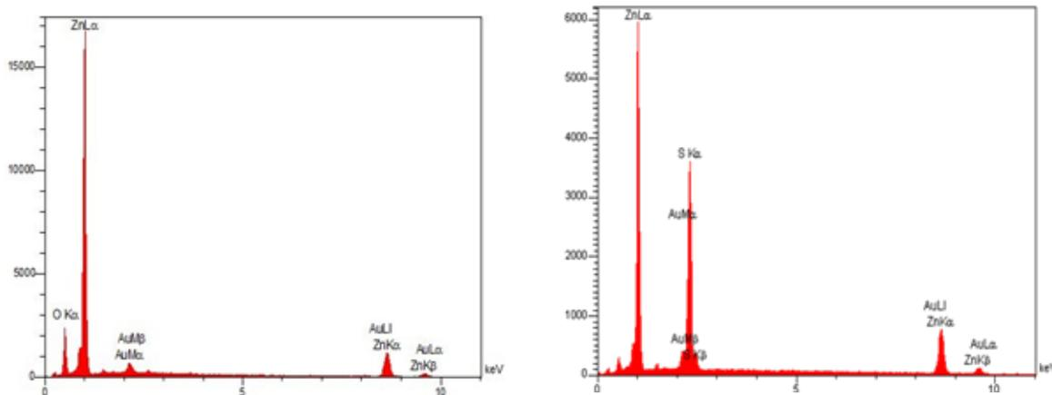
Figure 2: EDAX profile of ZnO nanoparticle (left) and ZnS nanoparticles (right).
