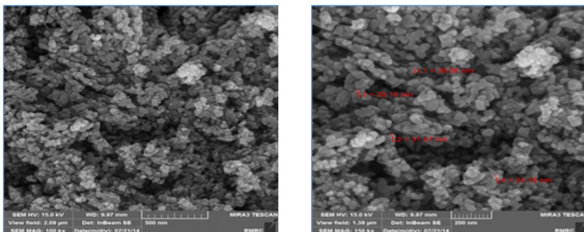
**Figure 1: Electro micrographs of ZnS (left image) and ZnO (right image) nanoparticles (100k magnitude)**
