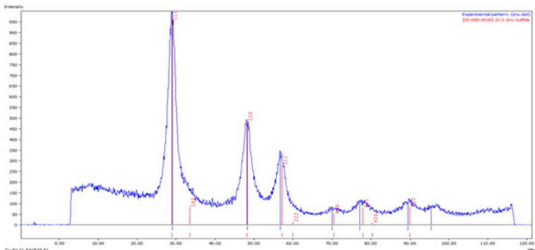
Figure 3: XRD curve of ZnS nanoparticles
